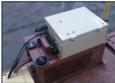
NEMA weather resistant housing contained RFID reader units, DC and/or AC power supply, cell communication and data interfacing control units.
