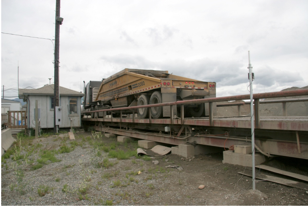
Figure 3: Granite scale in Anchorage with stationary pole and RFID reader/antenna in the foreground. The PaveTag™ processing hardware is the gray box sitting on top of the concrete support, next to the antenna pole. Photo by Janet Burton, University of Alaska.
