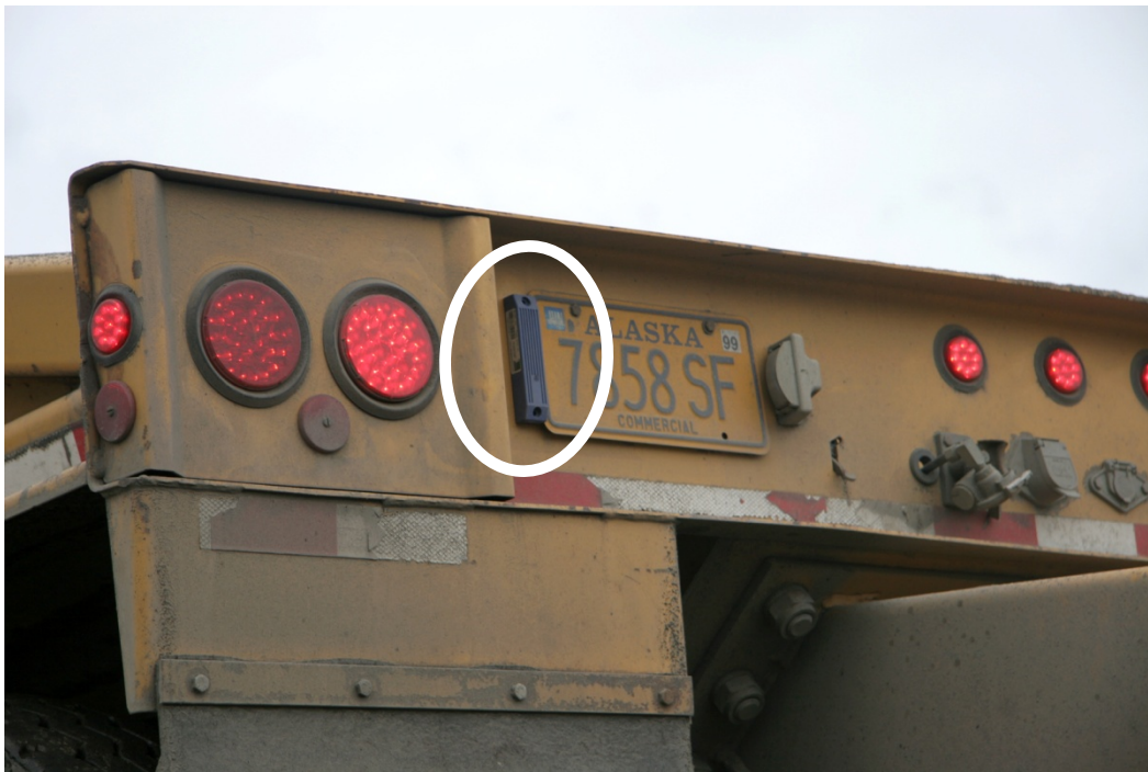
Figure 2: RFID Tab Mounted on a Hauling Truck (adjacent license plate - left side).
