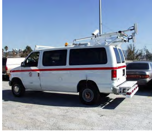
Fig. E.2 Semi-Automated Survey Van
