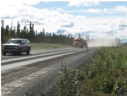
Figure 4 –Section 3A – 7/18/2011 –One day after application of Durasoil . (Note the difference in levels of dust generated by the two vehicles traveling at the same speed)
