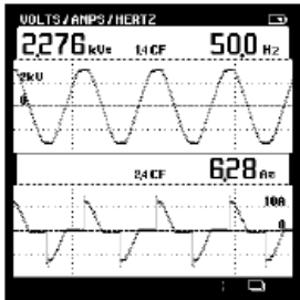
Voltage and current waveforms True-rms voltage and current Frequency
